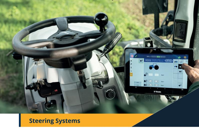
A wide selection of automated and assisted vehicle and implement steering systems from Trimble ensures maximum precision for all your farming operations. Hands-free guidance keeps your equipment on line no matter the field pattern or driving conditions, while increasing safety through reduced operator fatigue.
