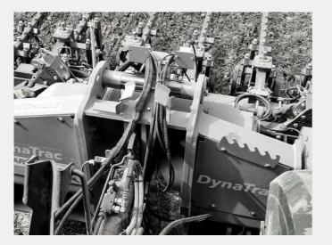
• Laforge offers an interface wich ensures repeatable and accurate implement positioning, regardless of the operation performed
